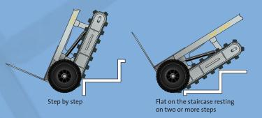
The SR Express is designed for a one man operation. It features several operator friendly functions and options including fast removable battery packs, remote control, different types of wheels, height adjustable platform and adjustable handles.
